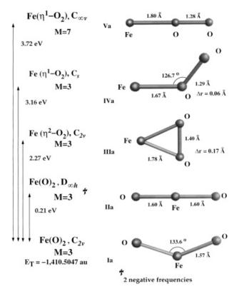
**FIGURE 2.** Structural parameters and relative energies calculated by geometry optimizations for the lowest energy states for Fe(O)<sub>2</sub>,  $C_{2v}$ ; Fe(O)<sub>2</sub>,  $D_h$ ; Fe( $\eta^2$ -O<sub>2</sub>),  $C_{2v}$ ; Fe( $\eta^1$ -O<sub>2</sub>),  $C_s$ ; and Fe( $\eta^1$ -O<sub>2</sub>),  $C_v$ , at the LSDA-VWN level of theory.
